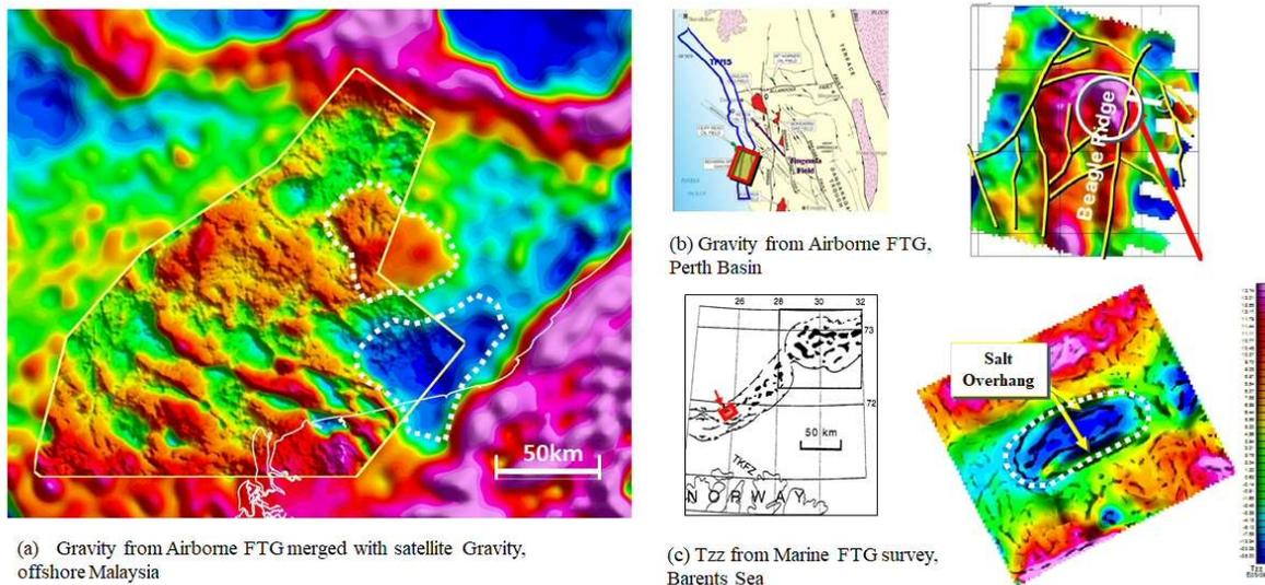
Figure 1. Data examples of FTG. (a) merged gravity from FTG with satellite data mapping regional geology, (b) focussed gravity from FTG defining structural block in Perth Basin and (c) FTG tensor analysis defining salt body shape in the Barents Sea, offshore Norway.
